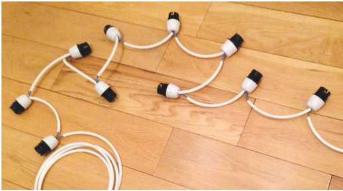
▲ Pic.11 Before you start this step, it's very important to know what you're doing, and I recommend consulting a professional. Wiring up the lamp involves lots of safety considerations, so you need to be clued up before you start. All 11 lampholders had to be wired together in order for the lights to work, so starting at the one furthest from the plug, I began working my way along. Since there was roughly a 150mm gap between each lampholder on the MDF, I just cut 10 lengths of flex at around 250mm; this allowed extra wire for stripping and insertion into the terminals at the back of each lampholder. In the photo here you can also see that I added enough length to attach a plug
